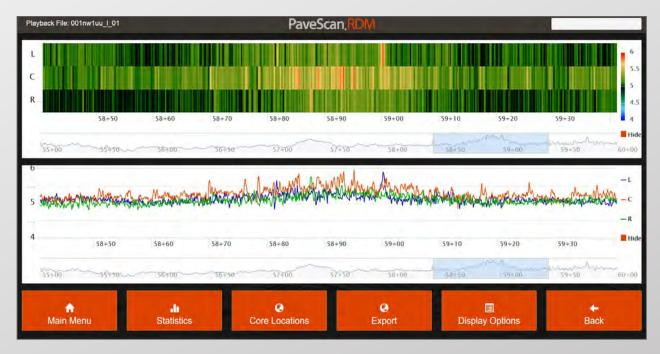
Data represents the visual output of PaveScan data. The color map indicates anomalies in the dielectric measurement. The line graph denotes the dielectric output of each sensor.
